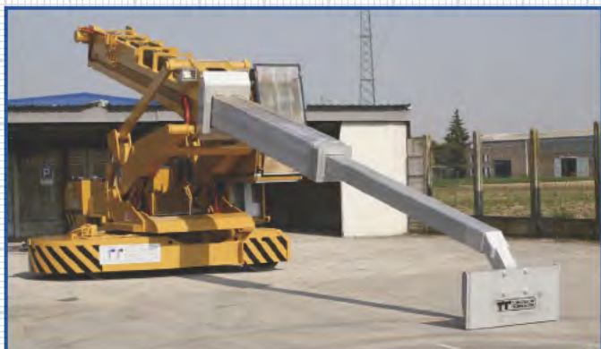
Special Skimming and cleaning vehicle equipped with 12 mt telescopic boom
