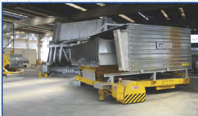
Automatic charging equipment with charging box of 12 m3.
